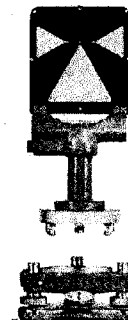
Fig. 11 Target GZM5 removed from the tribrach
